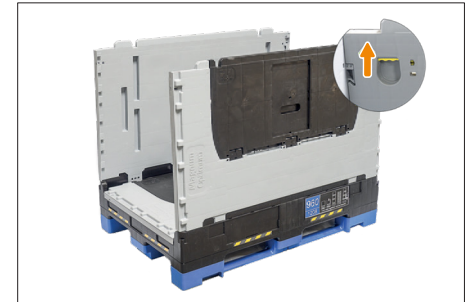
6. Unlock the second short sidewall from the long sidewalls and fold it down. The unlocking mechanisms are located inside of the box on the short sidewall.
